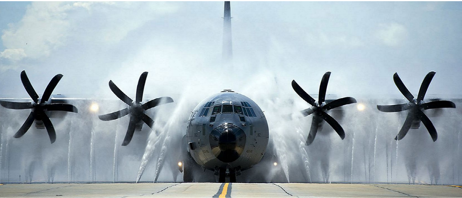
Dowty, a GE Aerospace company's R391 propeller has powered the Lockheed Martin C-130J Super Hercules in conjunction with the Rolls-Royce AE 2100 turboprop since 1994
